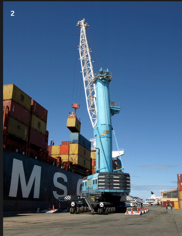
1. P&H 625OTC Truck Crane, purchased from Auckland, which was used on the early container ships 2. The Liebherr 320 Mobile Container Crane in action - this was purchased second-hand from PrimePort Timaru
