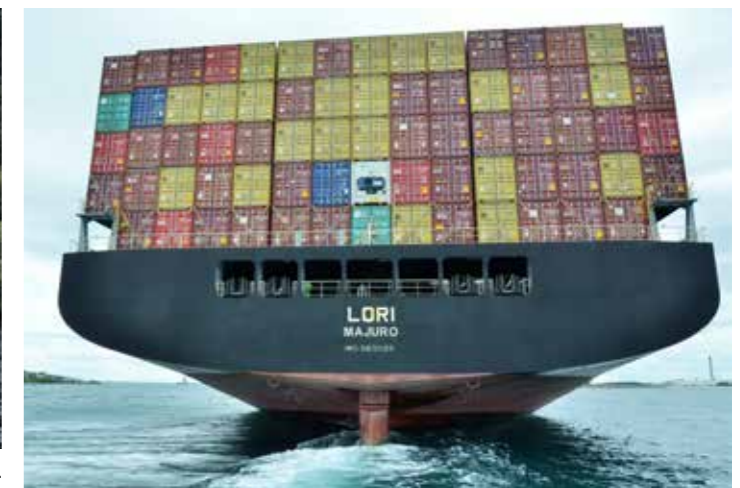
► Her 37 metre beam allows the Lori to fit 15 rows of containers across her upper deck.
