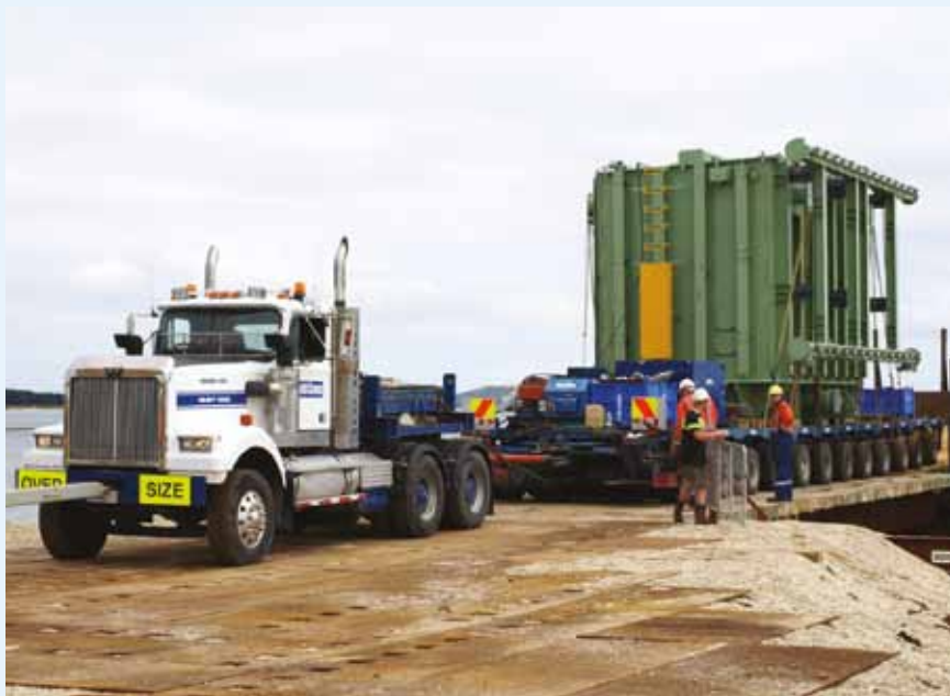
The transformer being inched ashore at Tiwai.
