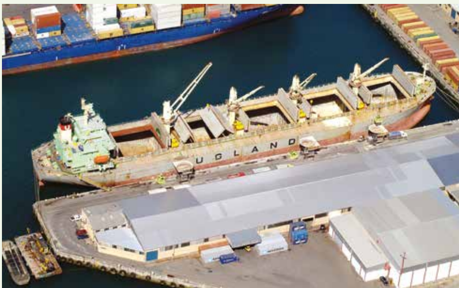
This aerial view of "Fermita" shows virtually empty holds as discharging of her fertiliser cargo nears completion.
