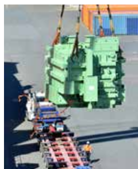
► COVER: Our cover photograph shows the generator ex Shansi being landed to road transport utilising the ship's cranes.
