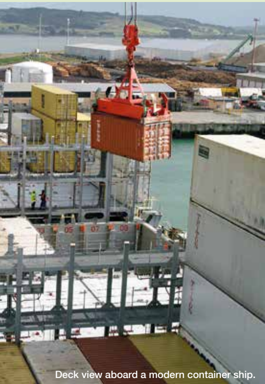
Corner posts are strengthened allowing containers to be stacked and mechanically locked together.
