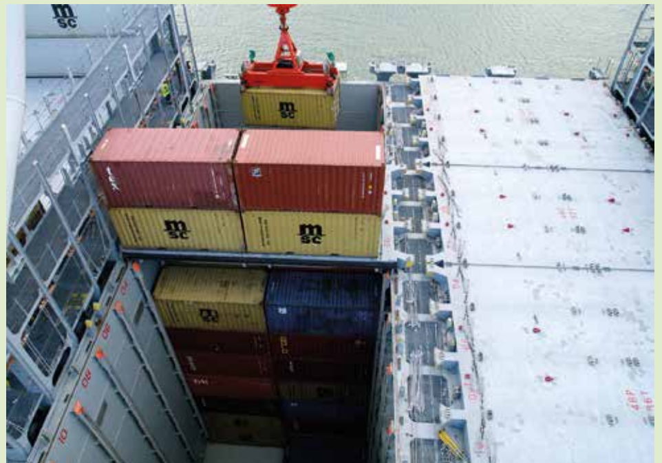
Illustrating why container ships are described as cellular.
