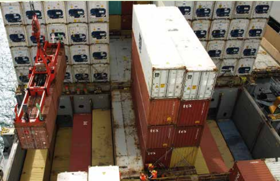
Containers in stow. The numerals across the after end are cell numbers, odd numbers to starboard (right), even to port (left), and those at the side are bay numbers, odd numbers for 20 footers, even numbers for 40's.
